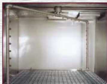
(Standard) Rotating blast pipe system
